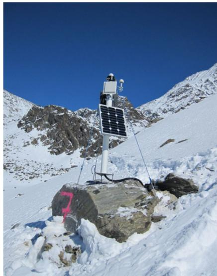
*Figure 3. 5: Example of a self-sufficient GNSS monitoring station of ETH Zurich, located in the Swiss Alps.*
