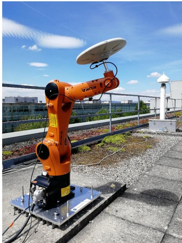
Figure 1. 53: Six-axis industrial robot KUKA KR 6 R900 sixx for GNSS receiver antenna calibration. The GNSS antenna in the back is the reference station.
