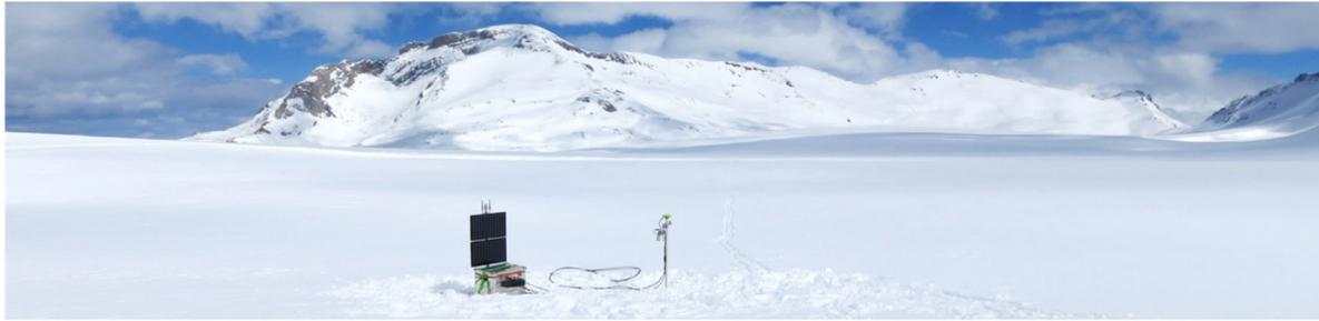
Figure 4. 12: GPS-reflectometry station at the Glacier de la Plaine Morte.
