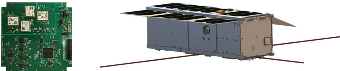
*Figure 4. 6: GNSS payload board (left) and Astrocast-01 satellite (right) with GNSS antennas located on top and on front face.*
