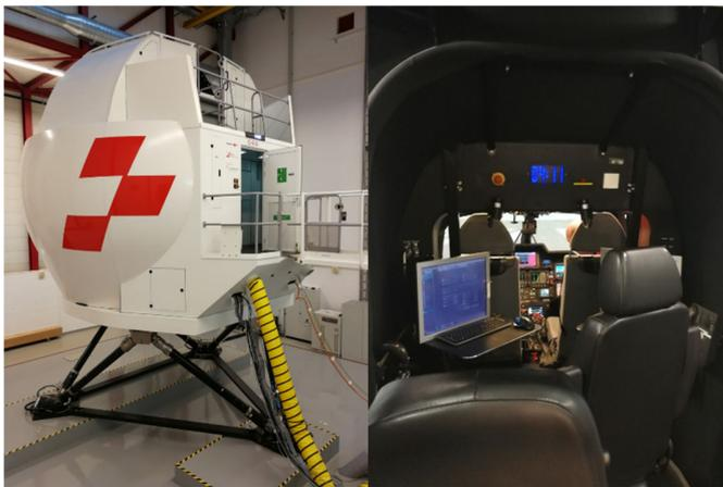
*Figure 4. 52: Full simulator at REGA's training center: A path, resulting from this optimization process, was entered into a full flight helicopter simulator. First simulator test flights proved the practicability of the results.
