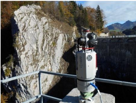
Figure 4.50: 3D terrestrial laser scanner
