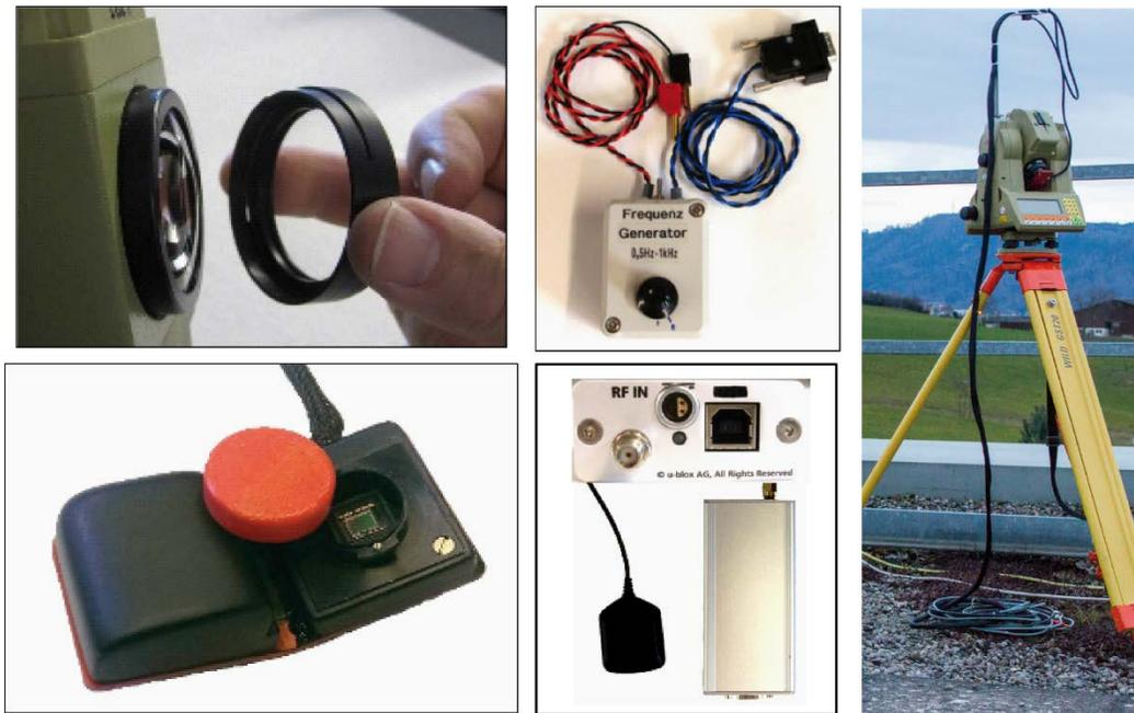
Figure 4.85: Main hardware components of the QDaedalus system.
