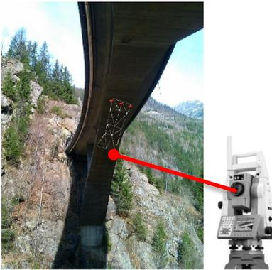
Figure 4.49: tacheometric measures with reflectorless techniques
