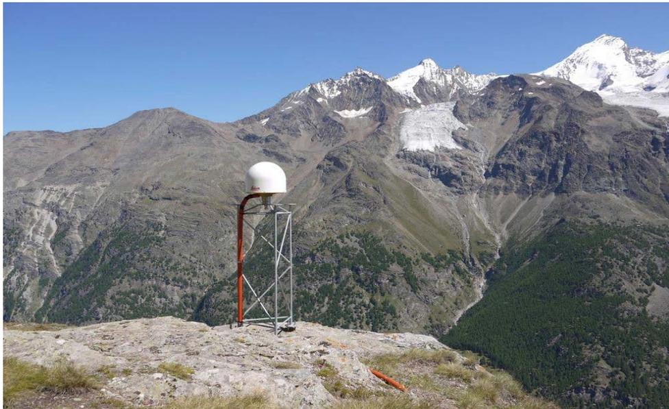
*Figure 3.13: Reference station RAND of the COGEAR GNSS network.*
