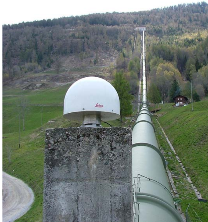
Figure 4.31: GPS permanent station for the monitoring of hydraulic infrastructure.
