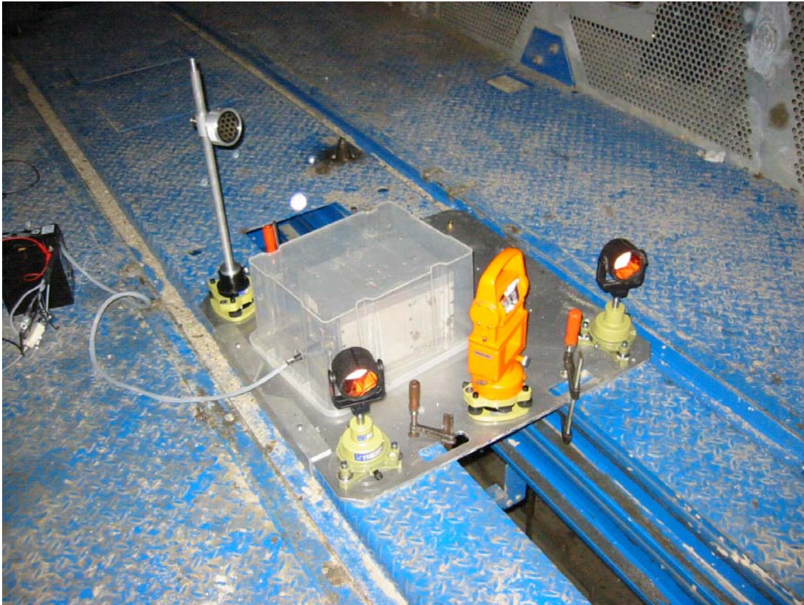
Figure 4.36: The INS and the autocollimation mirrors fixed in the mine cage.
