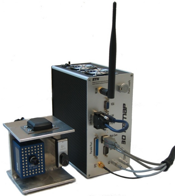
Figure 4.9: Preliminary version of a stand alone 3D capturing system "remap". Due to the concept it can be mounted on a robot which works in contaminated environments.
