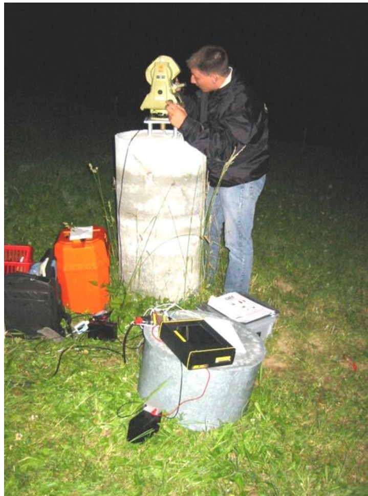
Figure 4.53: Student observing an astronomical azimuth near the Alptransit construction site Sedrun, Canton Grisons, Switzerland. The on-line measuring system ICARUS/AZIMUTH enables an automated measurement regime. The computer steers the total station (Leica TCA 1800), a dedicated GPS time receiver, and calculates the results of the observations in real time.
