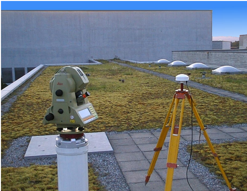
Figure 4.54: Astro-geodetic observation system ICARUS/AZIMUT. A Laptop computer and a small interface box complete the low-cost system which enables the determination of astronomical latitude, longitude, and azimuths in real-time.
