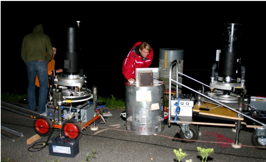
Figure 4.20: The two digital zenith camera systems TZK2-D (University Hannover, Germany) and DIADEM (GGL, ETH Zurich, Switzerland) observing at Amsteg, Canton Uri, near the portal of the 57 km long railway tunnel AlpTransit under the Swiss Alps in Central Switzerland. With these systems, deflections of the vertical can be determined with an accuracy of \leq 0.1 arcsec. Thanks the digital imaging technique, and the fully automated observation procedures, the results can be processed in near real-time.
