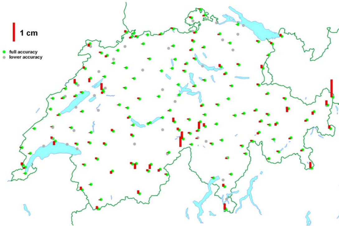
Figure 1.14: GPS height residuals of the combined adjustment CH-CGN (orthometric heights LHN95, geoid model CHGeo2004, GPS heights CHTRF2004).
