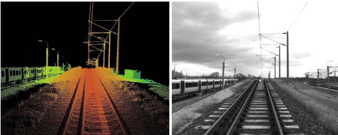
Figure 4.16: Comparison of a swiss trolley point cloud and the corresponding synchronised image. The high spatial resolution of the scan data allows for the contact-free, geometrical determination of the overhead line. The colour coding represents distances from the track axis.
