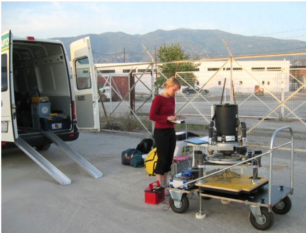
Figure 4.52: Instrumental transport and setup of DIADEM by means of a special trolley and electromechanical cylinders. These allow to lift up and lower the whole instrument. For recently performed observations and results, please refer to the contribution in section 2, page 47.
