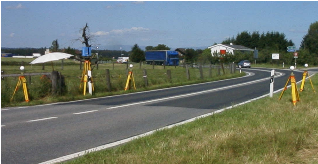
Figure 4.11: Measurement setup along the road area to be investigated. One can see the laser scanner and some tie points mounted on tripods. Typical vehicles are trucks and cars passing by in high frequency.
