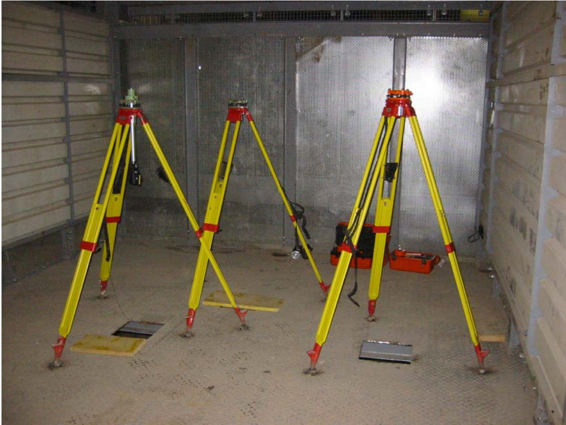
Figure 4.37: Optical plumbing installation in the mine cage at the top of shaft 2.
