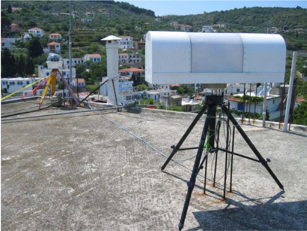
Figure 4.45: Instrumental setup of the radiometer (foreground) and the solar spectrometer (GEMOSS) at Alonnisos (Greece) during the validation campaign Jason-1.
