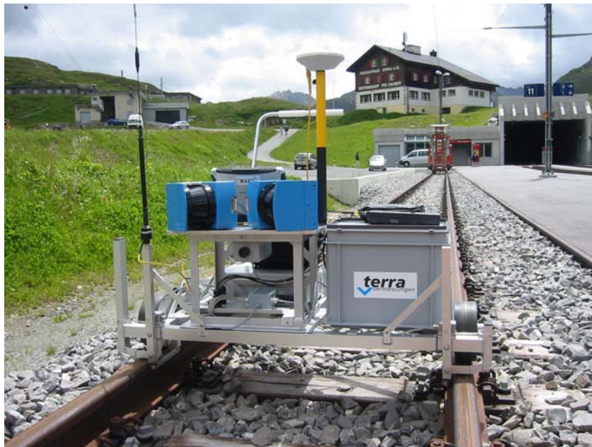
Figure 4.14: The metre gauge version of the swiss trolley . For positioning and attitude determination, differential GPS and inclination sensors are used. As an alternative on stretches without GPS reception, tracking totalstations can be applied. Two laser scanners generate fans skewed by 45^\circ with respect to the track axis. By the forward motion of the measuring system, a three-dimensional point cloud is generated. Additionally, an industrial camera provides every second a high resolution image.
