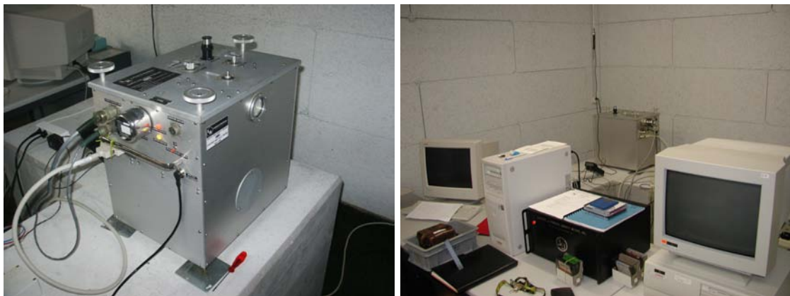
Figure 2.7: Permanent gravimeter ET25 in Zimmerwald.
