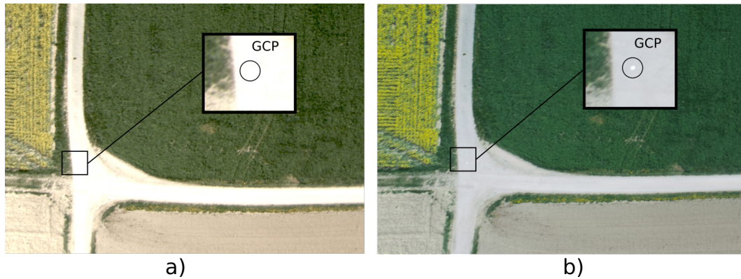
Figure 7.2 – Automatic and manual image conversion from raw to JPEG format; a) automatic conversion using the senseFly eMotion2, b) manual correction using a photo editor. The image was taken with the Canon PowerShot S110 camera having 12.1 Mpix resolution (Canon Inc. [2016]).
