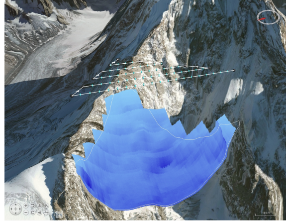
Figure 3.11 – Evaluation of GSD. The darker the blue colour, the lower expected GSD (Pascale [2016]).
