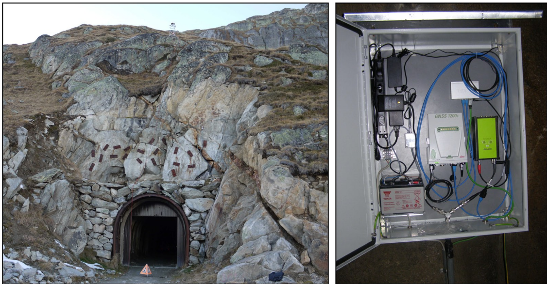
Figure 8.4: Left the Leica AR25 GNSS antenna at the station FIES is mounted over the tunnel, where the GNSS receivers and the broadband seismometers are installed. The Leica GRX1200 and Javad Sigma-G3TAJ GNSS receivers are connected via a splitter to the same antenna and are placed inside the tunnel (right).
