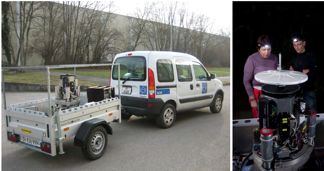
Figure 8.5: (Left) The astrogeodetic system DIADEM installed on the trailer for the field experiments at CERN. (Right) Monique Dupont (CERN) and Sébastien Guillaume (ETH) during a DIADEM data acquisition.
