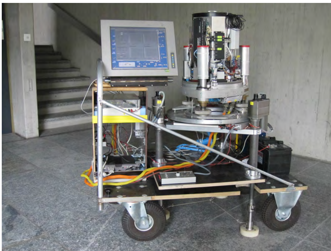
Figure 7.4: The Digital Astronomical Deflection System DIADEM in its last version (2014).
