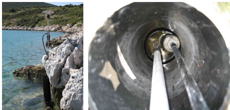
Figure 8.6: Left: Pressure tide-gauge station PELAN, with GPS antenna for the determination of absolute position and height. Right: view of the pressure gauge inside the tube.
