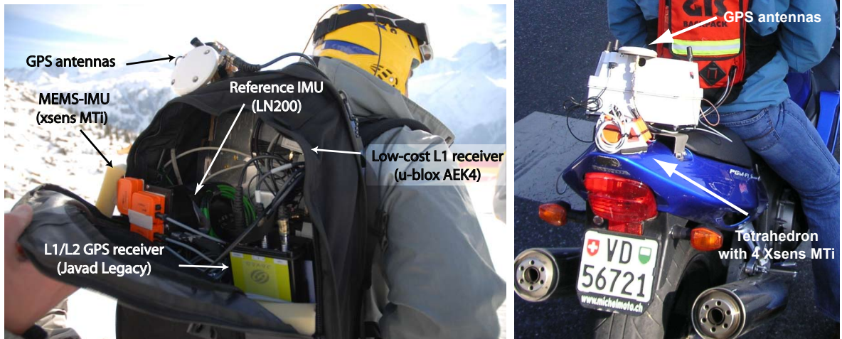
FIG. 4.2: Experimental setup mounted on a professional skier and on a motorcycle.
