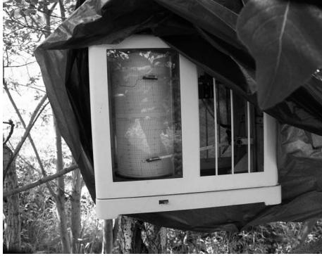
(a) Mechanical thermo-hygrograph installed nearby the GPS station GRIM (see Figs. 4.3 and 4.4 for the geographical location) protected from direct solar radiation and rainfall.
