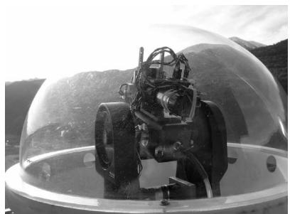
(a) The rotating sensors of the Geodetic Mobile Solar Spectrometer GEMOSS are protected by a transparent dome.
