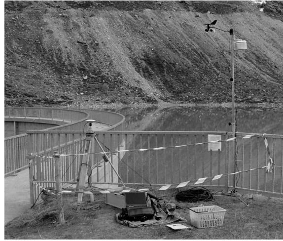
(b) Weather station of David Instruments (on the right hand side), mounted on the shore of the storage lake of Turtmann next to the GPS station SSTU (Leica System 500) (for the geographical location see Fig. 4.3 and the satellite visibility is given in Fig. 4.6(a)). The GPS antenna is put on a standard wooden tripod.
