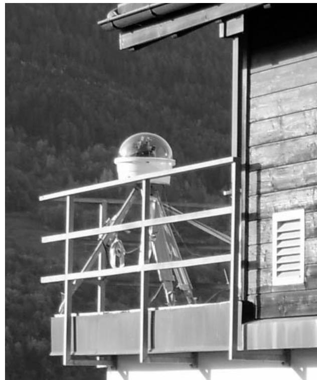
(b) Installation of GEMOSS on the terrace of the house. The GPS station HOHT of the AGNES network is mounted on its roof.
