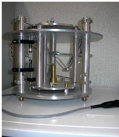
Figure 4-15: Small damping table of micro-g solutions (Height: 50 cm)
