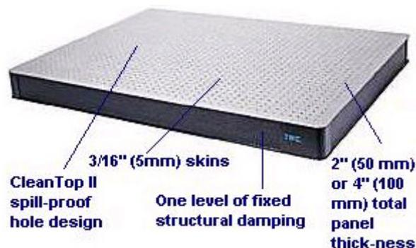
Figure 5-4: Optical table “Clean Top II” from TMC
