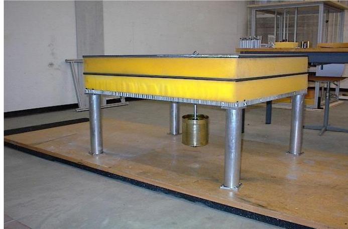
Figure 4-10: The experimental two layer absorbing table with its dynamic damper
