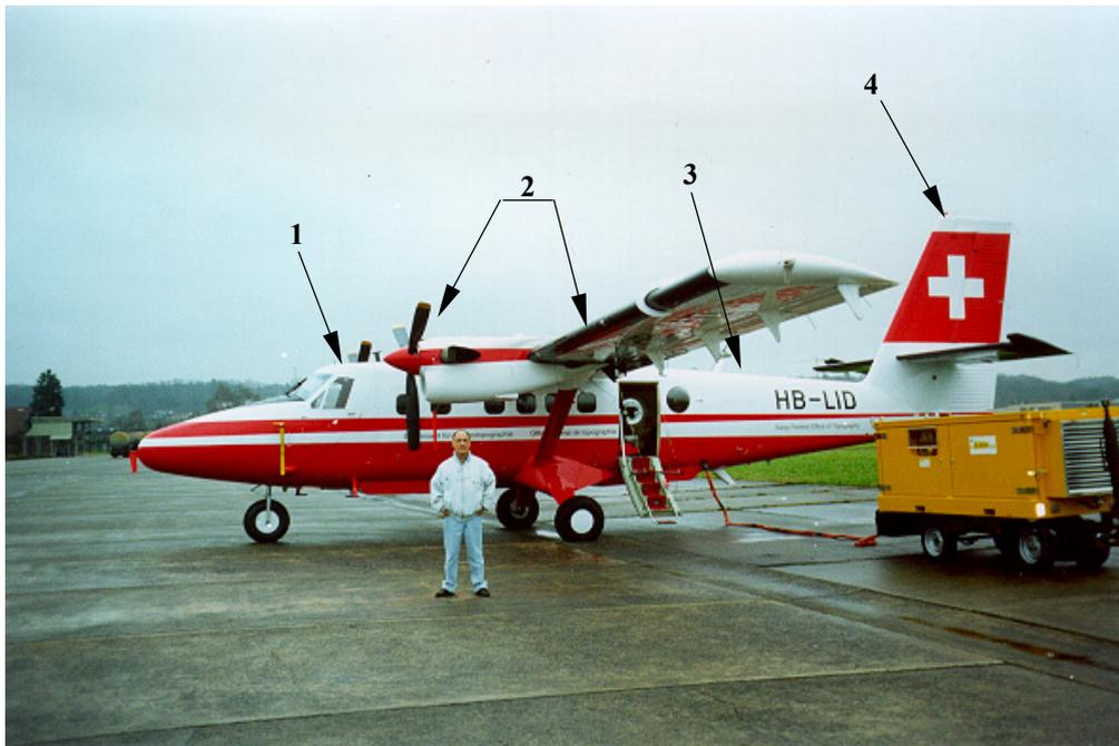
Figure 7-5: Locations of the *GPS* antennas on the aircraft. **1** : Front antenna (frnt), **2** : Wings antennas (left, rgth), **3** : Roof antenna, **4** : Tail antenna (tail)
