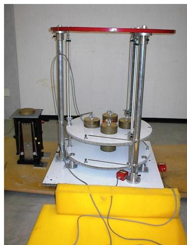
Figure 4-17: View of the experimental mounting used for the determination of the transfer function
