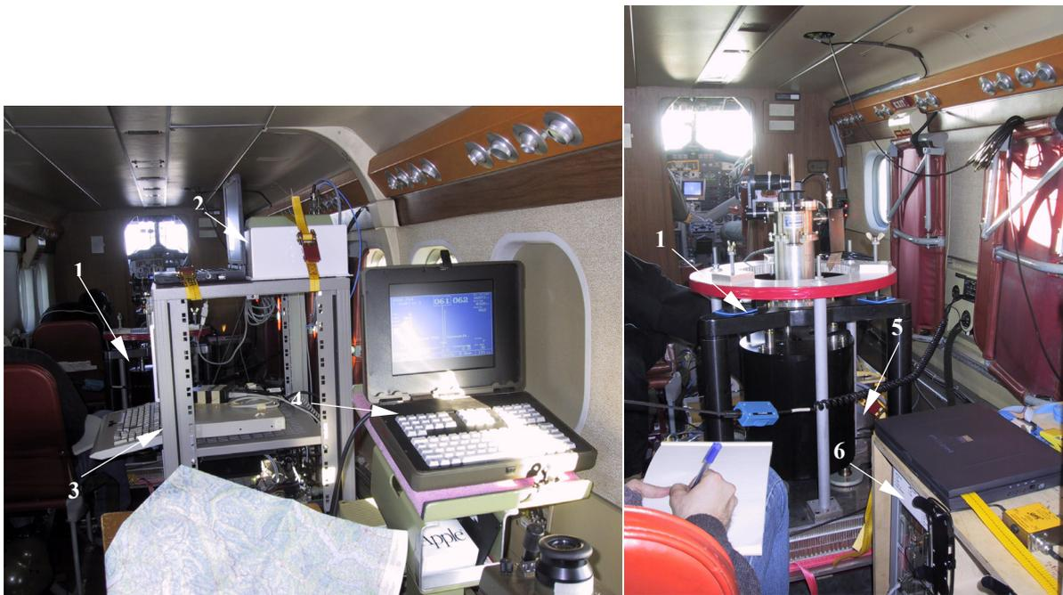
Figure 7-6: View of the interior of the aircraft during the test survey. **1** : Gravimeter FG5-L, **2** : Data acquisition system of the EpiSensor, **3** : Rack containing the GPS receivers and the PCs, **4** : Navigation system for photogrammetry, **5** : INS (Inertial Navigation System), **6** : Steering and data acquisition system of the l'INS.
