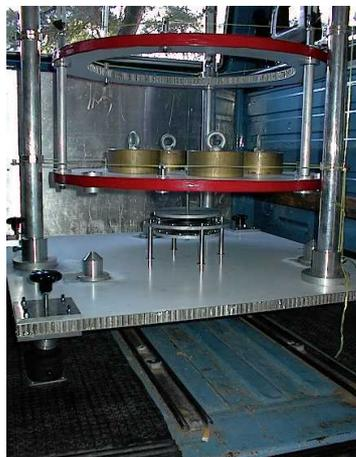
Figure 4-20: The last modified system mounted inside a small bus for the first dynamic test.
