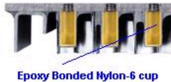
Figure 5-5: Structure of the body of the “Clean Top II” table
