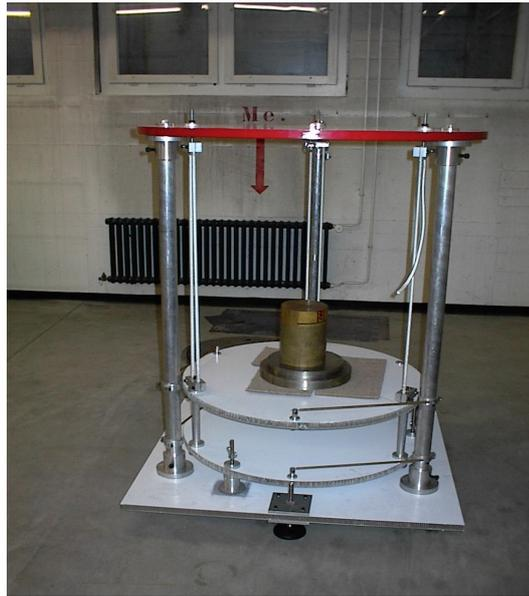
Figure 4-16: The first prototype of the table of second generation (Height: 180 *cm*)
