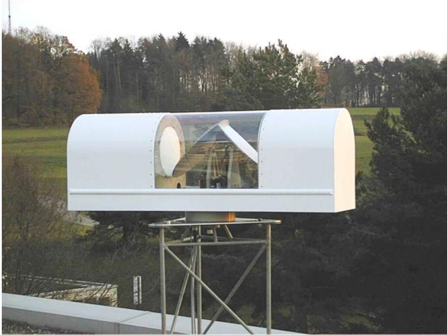
Figure 4.11: The new water vapor radiometer *WVR 2000* installed on the roof of the HPV building at ETH Honggerberg. Two mirrors reflect the radiation from the sky into two horn antennas.
