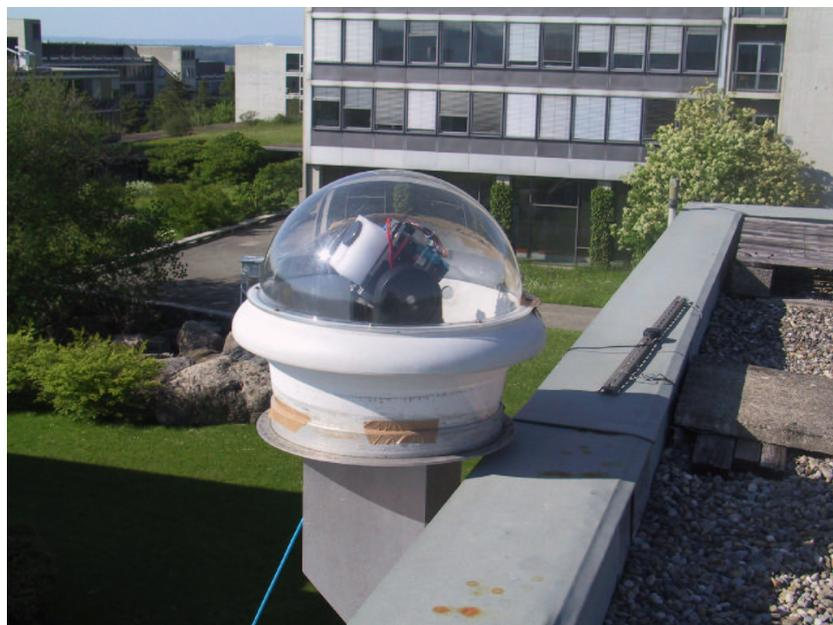
Figure 10.12: Sun-tracking telescope of GEMOSS installed next to the GPS station “ETHZ”. The glass dome protects the telescope against rain. The solar radiation is transmitted via an (blue) optical fiber into the spectrometer located inside the building.
