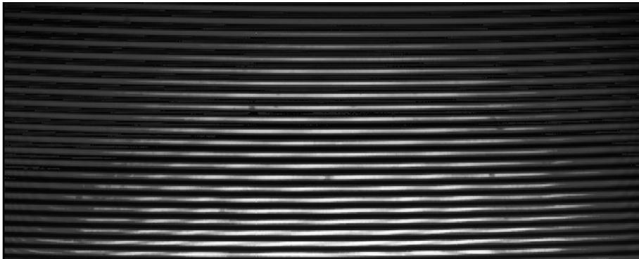
Figure 7.8: Image of a halogen spectrum measured by GEMOSS I. The approximate constant emission of radiation enables the determination of the polynoms describing the shape of the minima (black interstices between the white orders).
