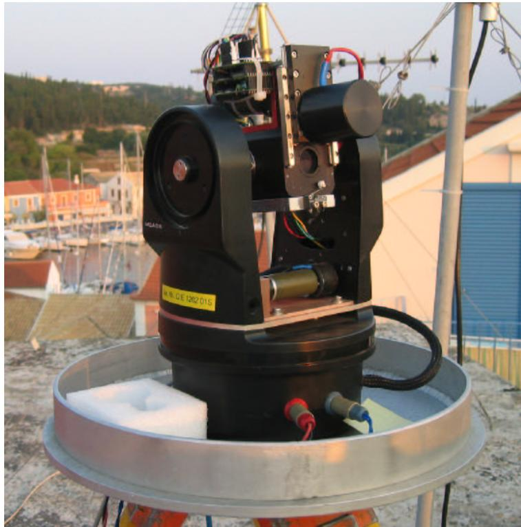
Figure 7.3: The telescope of GEMOSS I measurement system tracks the Sun using pre-calculated coordinates. A halogen lamp for calibration measurements covered by a black cylinder is mounted on a vertical slide.
