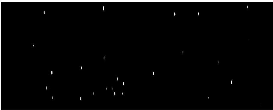
Figure 7.9: Image of a neon spectrum measured by GEMOSS I. The emission lines (white vertical lines) are used to correlate the pixels with the wavelength scale.
