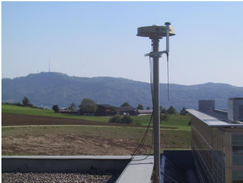
Figure 10.11: GPS antenna of the AGNES station “ETHZ” on the top of the HPV building of ETH Honggerberg.
