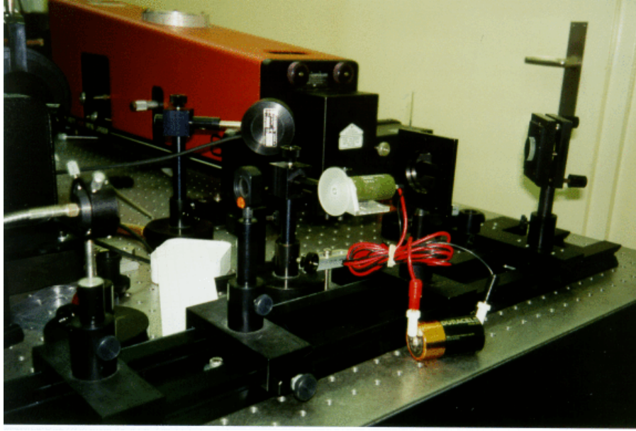
Figure 5.7: Setup for coupling the laser light into the SAMOS spectrometer. The beam is turned around by a mirror to pass through a perforated glass disk (white, in the center of the picture), which is rotated during the measurement. This destroys the unwanted coherence of the light, which falls onto the optical fiber to be conducted to the entrance slit.
