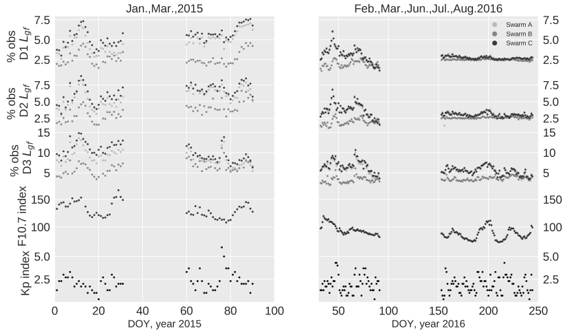
Figure 6.18: Percentage of screened position in comparison to the F10.7 and Kp indices.
