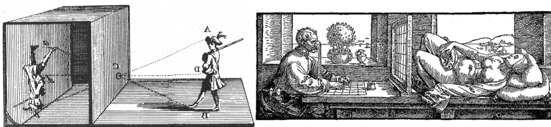
Figure 1.1. Camera Obscura Principle (left) and Perspective principle from an engraving by Albrecht Dürer (right). (For concordance with next images, the engraving have been mirrored horizontally)
