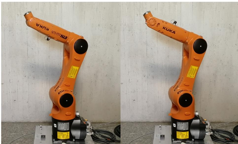
Figure 5.1.3 : The KUKA robot in two different postures but in the same pose (position and orientation of the flange).
