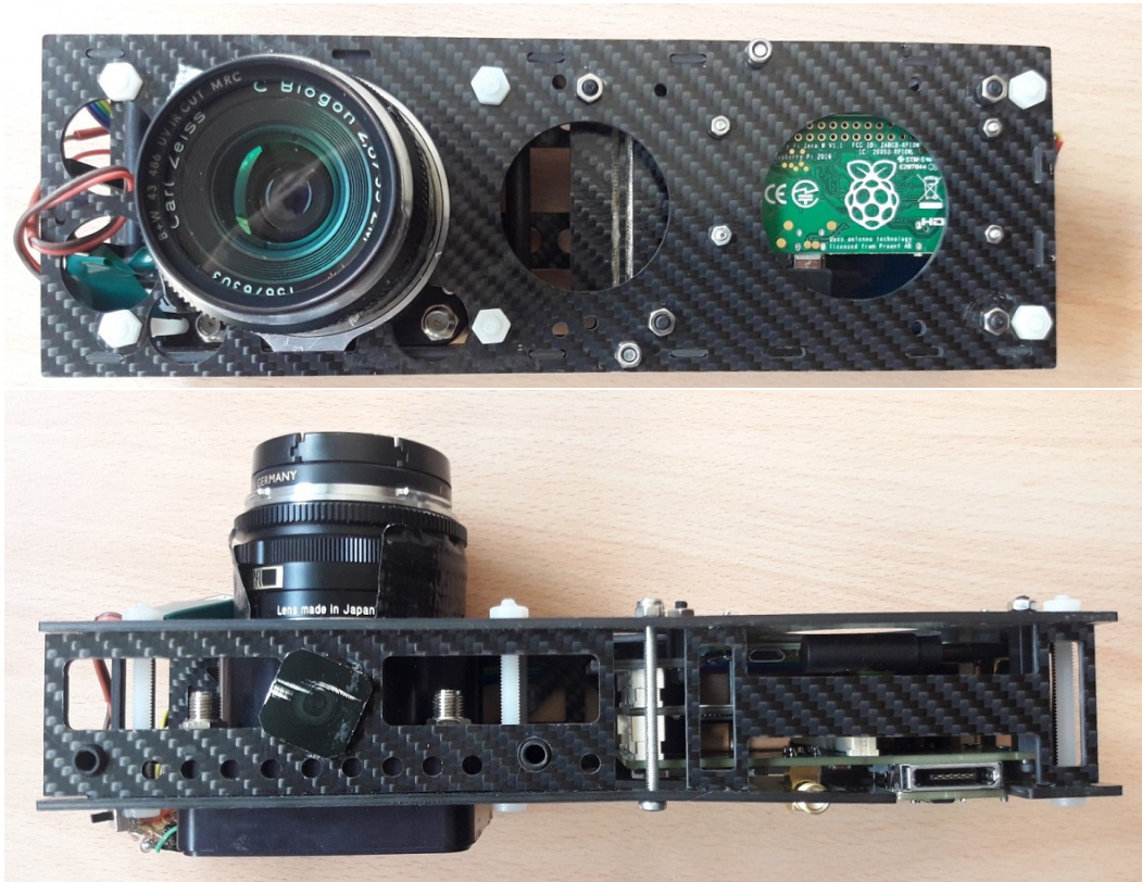
Figure 9.7: Bottom and side view of the IGN camera carbon mount (length of 23 cm) together with the IMU board and the embedded computer.
