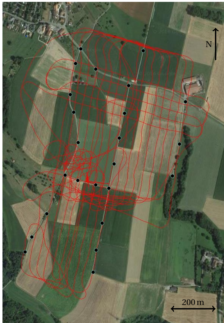
Figure 9.9: Test-site showing the flight path (in red) of the micro UAV with distribution of ground control points (black dots).
