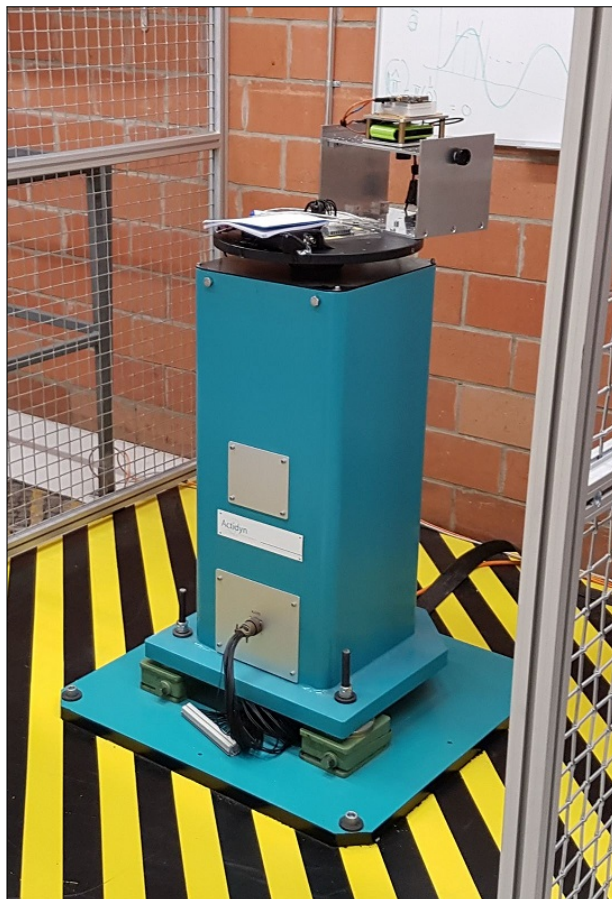
Figure F.1: Rotation table with 40 cm diameter base plate.
