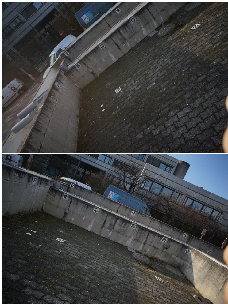
Figure 8.4: Example of 2 photos taken at different attitudes from the calibration field with the visible black/white targets.
