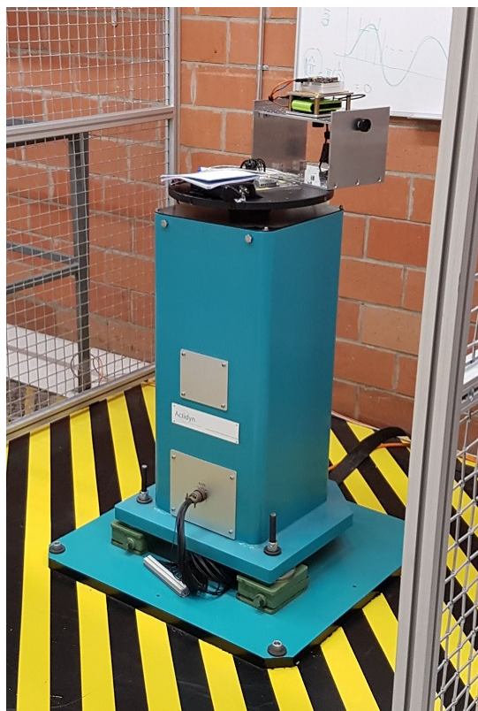
Figure 4.6: IMU installed on the one-axis high-precision rotation table (Appendix F).
