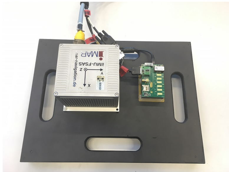
Figure 4.9: The 41 cm by 31 cm mount holds the IMAR and the Navchip sensors. The handles allow for easy grip and save manual swinging of the setup with the power and data cables leaving the platform.
