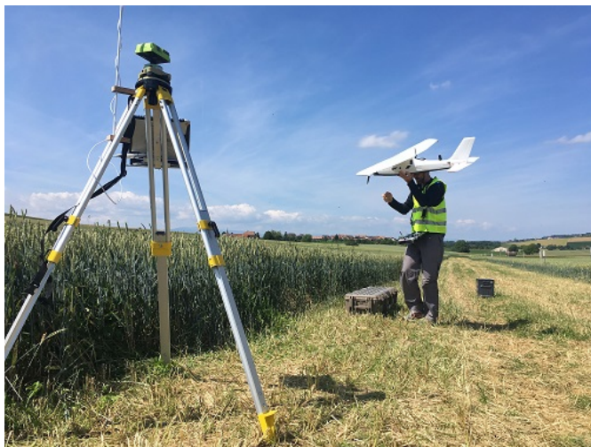
Figure 6.6: Typical test site for a UAV mission. The internal \mu PC of the drone is connected to the GCS via the WiFi-Link and transmits information about the calibration process during handling.
