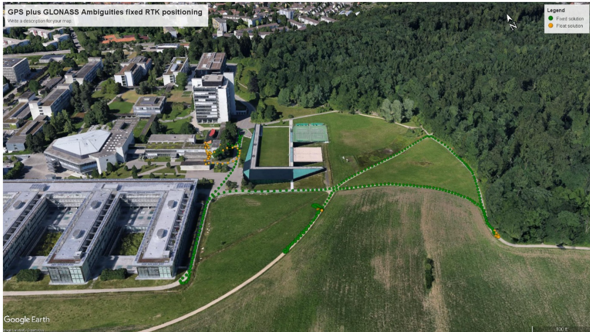
Figure 102 The bike route measured by the RTK positioning using GPS + GLONASS (both ambiguities fixed)
