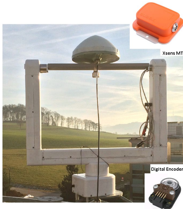
Figure 45 The rotating platform (with a Leica AR10 antenna connected to a Leica GR10 receiver)
