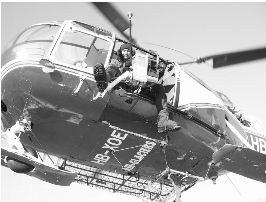
*Figure 1: EPFL's HELIMAP system in action augmented by LIDAR during a feasibility test, february 2004.*
