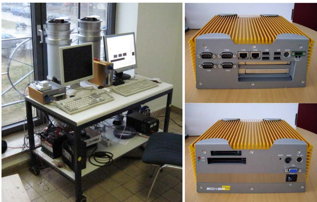
(a) Measurement Systems SOLUSAR I and SOLUSAR II set up at ISAS, Berlin with associated external components, such as computers and power supplies (underneath the table)
