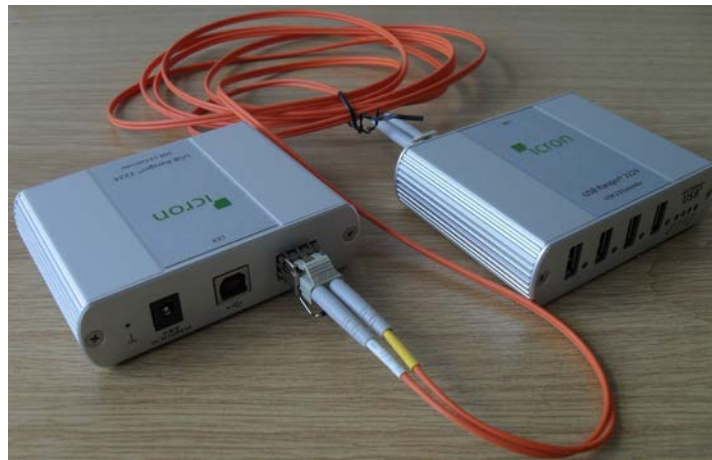
Figure 4.40: Icron USB-Ranger 2224. Data transfer between the various devices on the instrument side and the host computer is accomplished through conversion to optical signals and transmission via optical fibre. USB lines on the instrument side are bundled in a 4-channel USB-Hub (right device, powered by the car battery supplying the camera) and data conveyed via multi-mode fibre to the host-side device.
