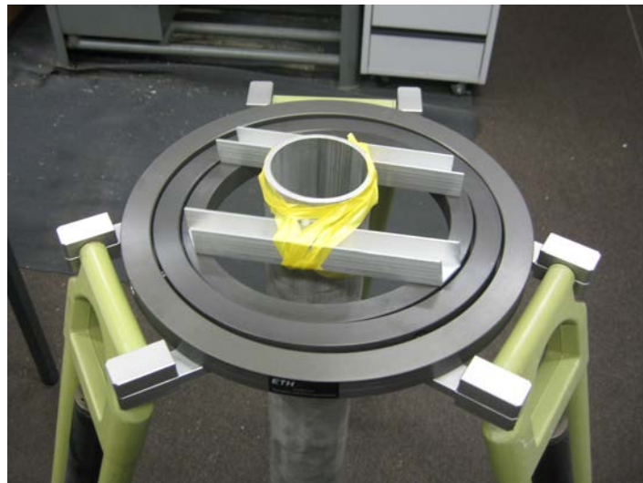
(b) Tripod with gimbal suspension for vertical stabilization of the instrument during deployment on moving platforms. In this picture the instrument is simulated by means of a vertical tube
