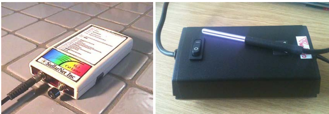
(a) StellarNet SL2 calibration lamp
