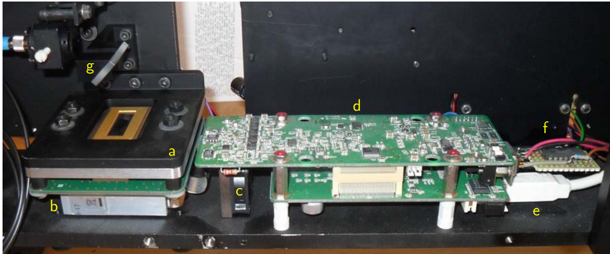
Figure 4.17: OEM CCD camera Hamamatsu C9260-933-17. The detector head (a) is temperature-stabilized by a Peltier element. The sensor head's heat sink (b) is supported by two small fans (c). The camera controller (d) is controlled via USB interface (e). For full galvanic insulation of the camera the USB signal is conducted via optical fibre to the main computing unit. The camera-generated shutter signal is transferred via optocoupler (f, compare Section 4.10.6). (g) denotes the folding mirror guiding the light from the spectrometer onto the CCD chip. The mounting plate of the camera is blackened as are most mechanical elements inside the spectrometer.
