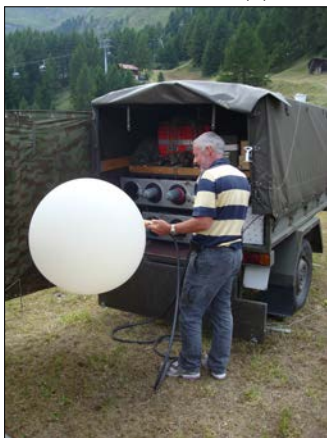
(b) Inflation of balloon with hydrogen.
