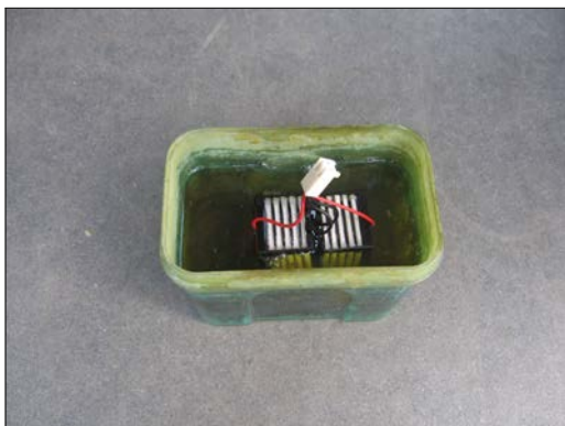
(c) Sonde battery in the water bath for activation.
