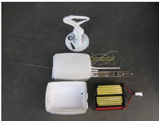
(a) From top to bottom: the attachment for the balloon, the sonde with the sensors, battery case and battery.
