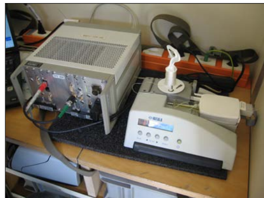
(b) Calibration set from Vaisala with the sonde being calibrated.
