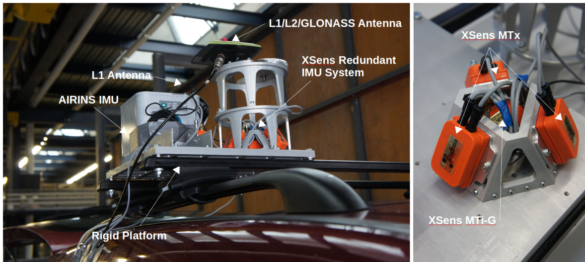
Figure 9.2: Navigation sensor platform mounted on the roof of the car (left picture) and view on the skew-redundant XSens inertial sensors forming the realized DIMU (right picture).
