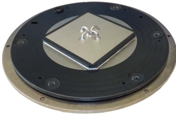
Figure 3.13 Geodetic patch antenna used in Trimble antennas. (Picture: D. Grimm)
