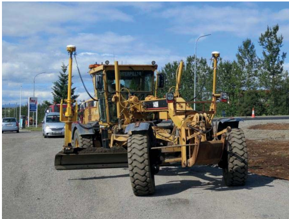
Figure 5.1 Grader with two GNSS antennas to control the blade. Picture (L. Steiner)
