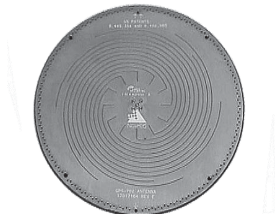
Figure 3.19 Pinwheel™ antenna for L1 and L2 modified picture from (NovAtel, 2006).
