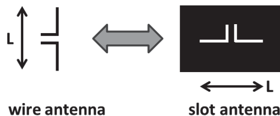
Figure 3.17 Babinet's principle applied to antennas.
