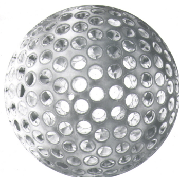
Figure 4.1: Illustration of the LAGEOS-1 sphere with its retroreflectors
