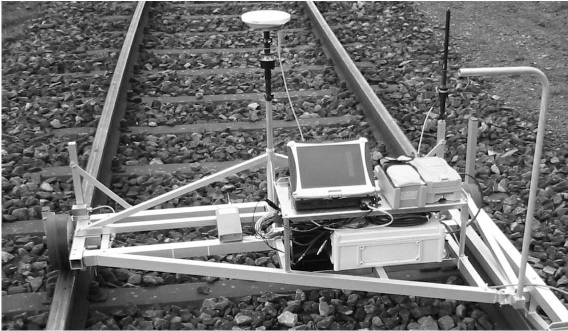
Figure 4-1 Track-surveying vehicle “Swiss Trolley” with a Trimble Zephyr antenna and a Trimble ATS600 active prism (P configuration)
