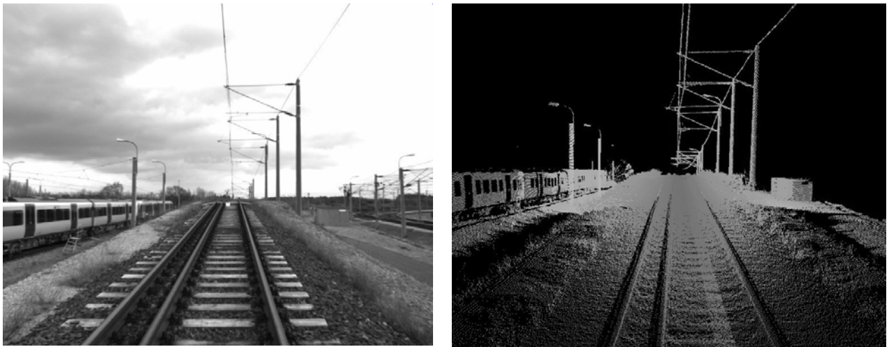
Figure 4-32 Kinematic scan of an overhead line. The overhead wire has a diameter of about 6 mm and is 5.7 m above the track axis.
