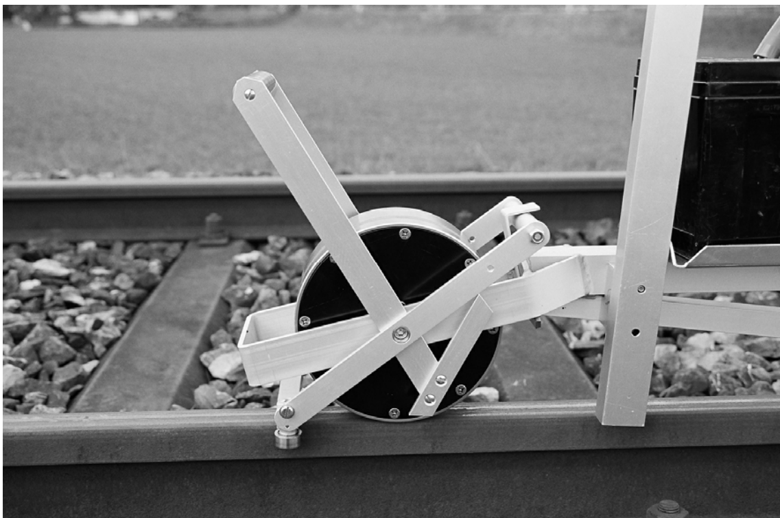
Figure 4-2 Back wheel with mechanism for passing switches
